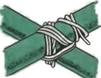
Diagonal lashing completed
