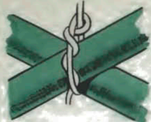
Timber hitch loose
